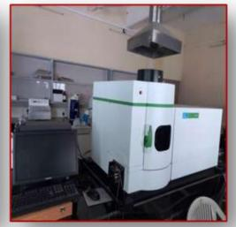
INDUCTIVE COUPLED PLASMA OPTICAL EMISSION SPECTROSCOPY
